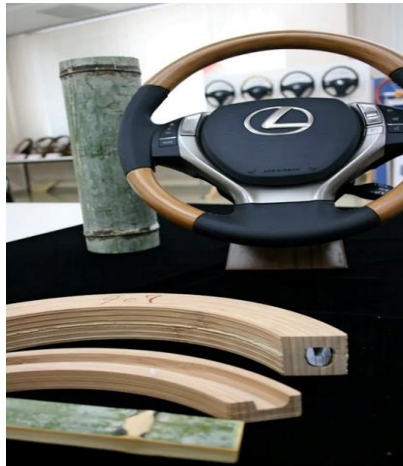
Figure 7. Steering wheel with antibacterial properties as a new bamboo product in Japan (Source: https://www.mirokutw.com/ )
